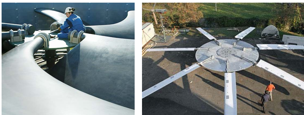
Figure 5: Large-scale rotors used for cooling towers
