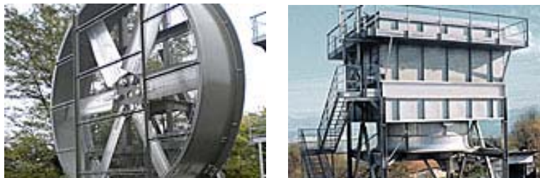
Figure 4: Example test rigs of a cooling tower fan rotor supplier
