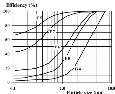
Many filters in operation, especially those with electrostatically charged filter material, never reach the average efficiencies used for classification and the Swedish National Testing and Research Institute require the following minimum efficiencies in a real life time test.
